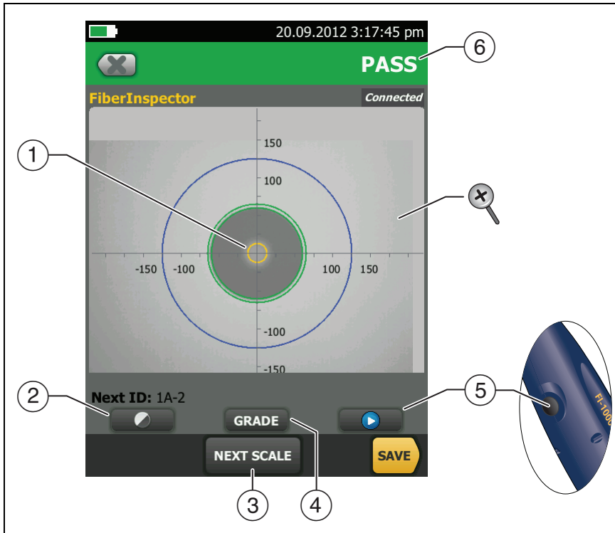
Figure 38. FiberInspector Image with Manual Grading Selected
