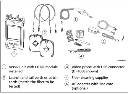
Figure 20. Equipment for FaultMap Tests
