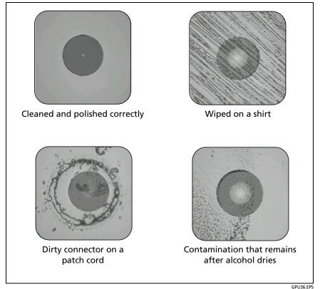
Figure 8. Examples of Clean and Dirty Fiber Endfaces
