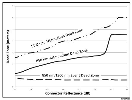
Figure 34. Typical Dead Zone Performance of Multimode Modules
