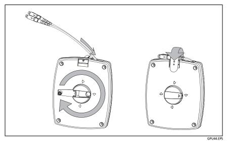
Figure 7. How to Retract the Launch/Tail Cord
