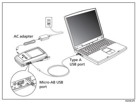
Figure 32. How to Connect the Tester to a PC
