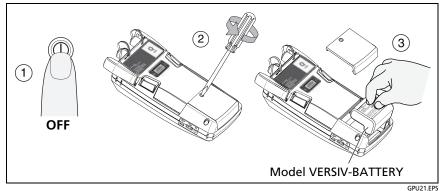
Figure 33. How to Remove the Battery
