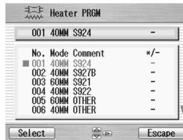
The S123 Fusion Splicer is installed the factory-set Heat Programs as follows.
