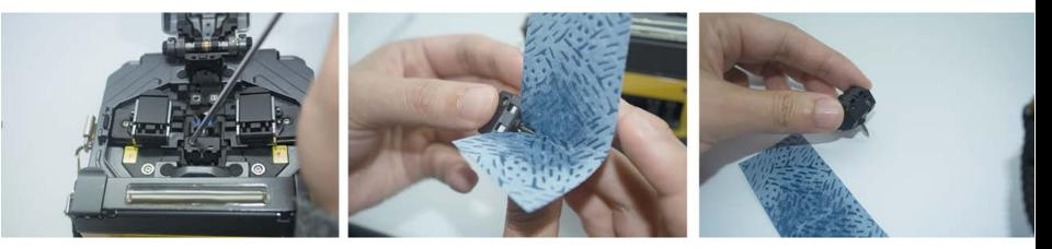
**4.** Remove electrodes carefully with a screwdriver
